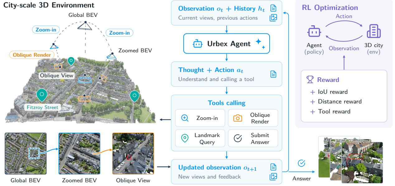
Figure 2 Architecture of Urbex: (left) a multi-view environment exposing global BEV, zoomed, and oblique views; (middle) the policy’s reasoning trace and tool calls over observation o_t and interaction history h_t ; (right) RL under a terminal reward (IoU and center-distance) plus tool-level shaping.
