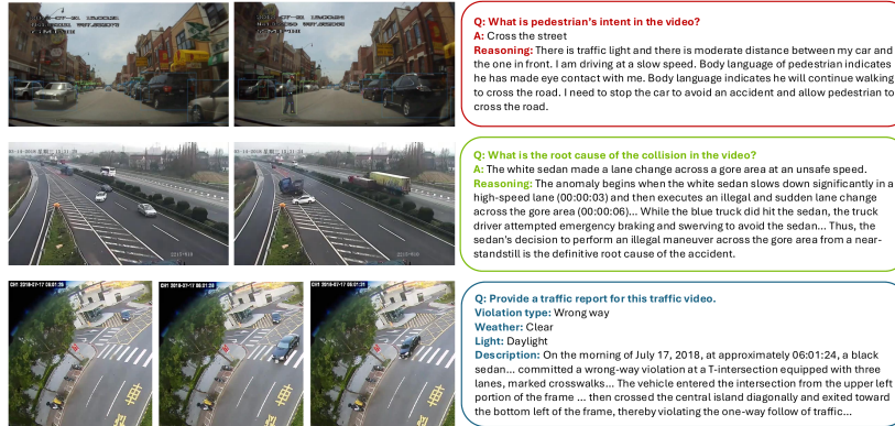
Fig. 3: Track 3 sample: traffic anomaly reasoning combines video evidence, task-specific questions, event descriptions, and causal explanations.
