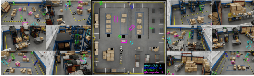
Fig. 1: Track 1 sample: synchronized multi-camera warehouse views and a top-down layout for RGB-only multi-camera 3D perception.
