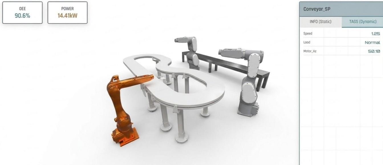
Figure 6. Live CDT dashboard: Real-time synchronization of industrial telemetry via MCP-enabled tool calls.
