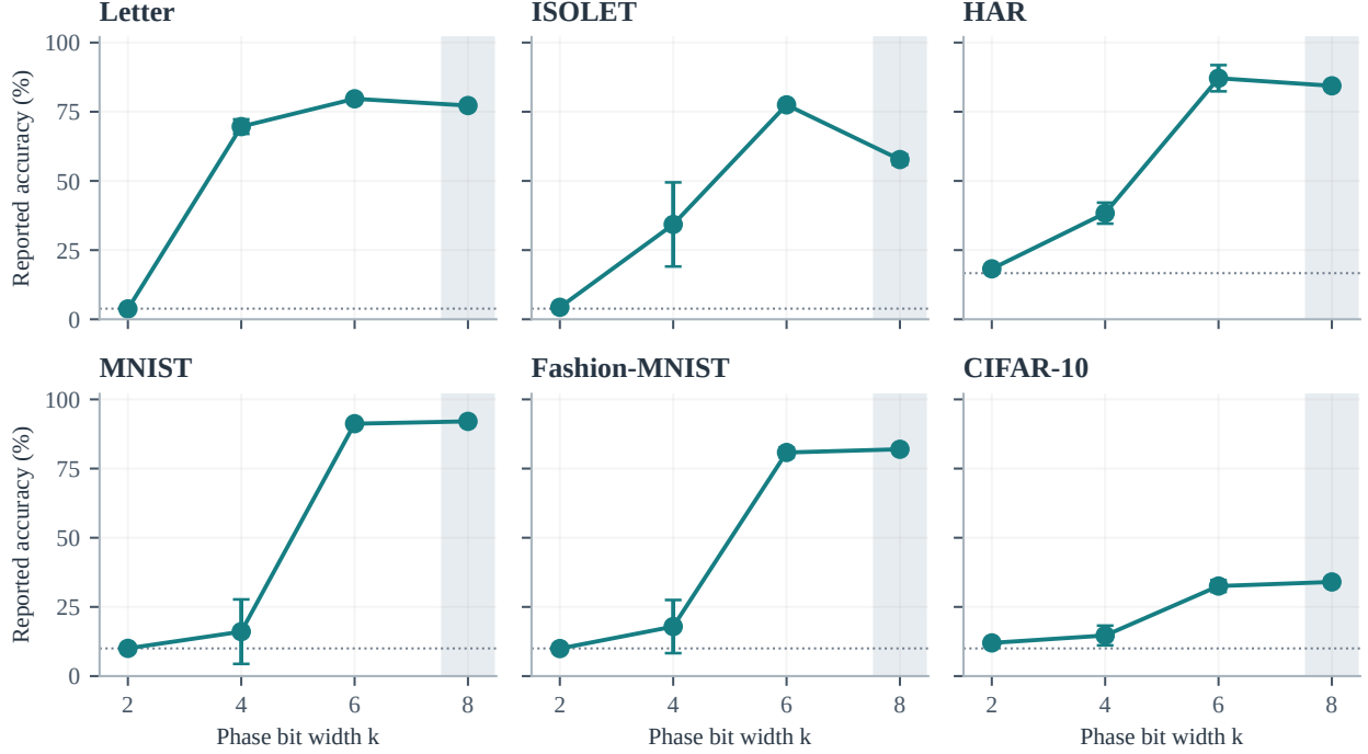
Figure 6: Phase-width sweep of Phase-HDC on six datasets. Mean accuracy and sample SD over three seeds. Dotted lines mark 1/C . The shaded column marks k = 8 , where the selected encoder threshold lies at the grid boundary on five of six datasets. Step size and effective gate change with k (Eq. (6)), so the sweep is not an isolated capacity experiment. Exact values are in Table 14.
