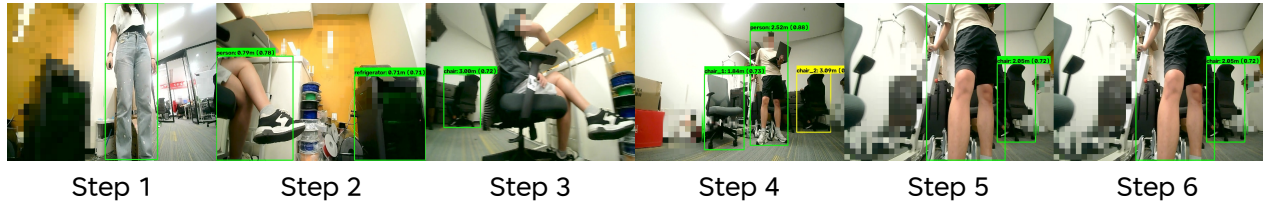
Figure 5 Visual search before greeting. The requested person is outside the quadruped’s camera view in steps 1–3, identified by clothing and laptop attributes in step 4, and seen at close range in steps 5–6. Frames follow the interaction from left to right; bounding boxes show object detections.
