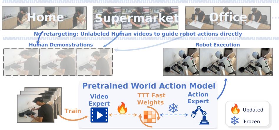
Figure 1: Overview of WAM-TTT. Given unlabeled human demonstrations from diverse environments, WAM-TTT steers a pretrained World Action Model (WAM) without retargeting, robot actions, or human-side annotations. During deployment, human videos are absorbed into lightweight TTT fast weights through self-supervised video prediction, while the pretrained action model remains frozen. The adapted memory then guides robot execution through the WAM’s shared visual-action dynamics, enabling efficient and reusable steering from human demonstrations.
