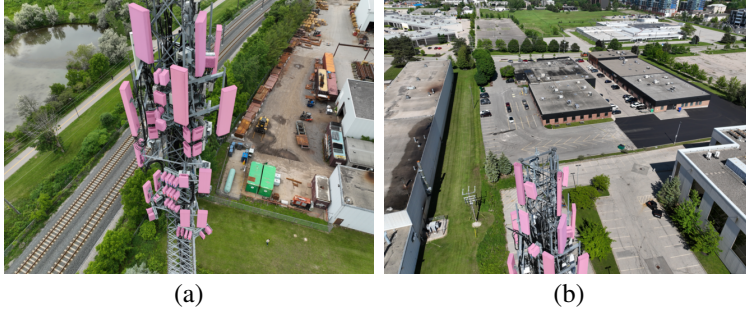
Figure 2: Representative instance-level annotations from TOW-300. All component instances are shown using the same overlay color (pink) for improved visibility and visual clarity.
