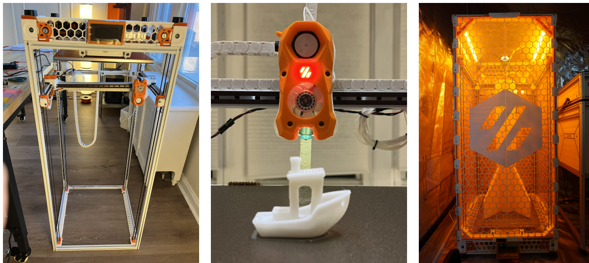
Figure 18: (Left) Voron-2-Tall during assembly, upside down to access internal electronics underneath the build plate. (Middle) First successful Benchy print with fully assembled printer and StealthBurner 59 toolhead using PLA filament. (Right) Voron-2-Tall with finished print for lower airframe component of Big Heavy 2 60 using ABS filament.
