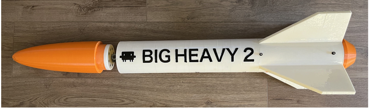
Figure 16: Recovered High Power 4 rocket in reflyable condition with minor cosmetic blemishes along the nose cone and lower airframe.
