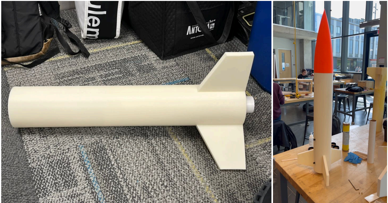
Figure 11: (Left) Lower airframe printed using ABS filament with motor tube inserted (Right) Initial completed assembly of rocket with post design installation of rail buttons.
