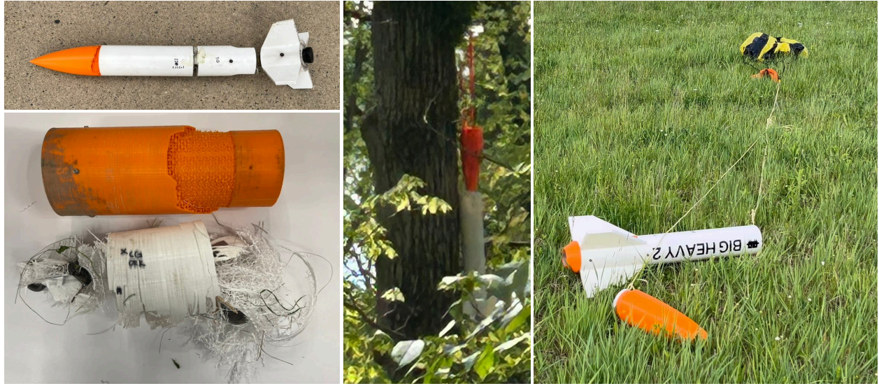
Figure 13: (Top Left) Recovered High Power 1 components after fracture from ejection charge (Bottom Left) Recovered High Power 2 components after recovery bay separation failure (Middle) Successfully recovered High Power 3 after landing in tree (Right) High Power 4 after successful recovery deployment and landing in field.
