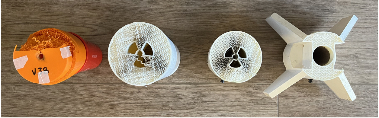
Figure 14: Recovered components of High Power 1 after successful launch including: (Left to Right) damaged nose cone with eyebolt removed post recovery, top section of lower airframe component with split at baffle section, middle section of lower airframe split between baffle and fin can, and bottom section of lower airframe including housing for electronics.
