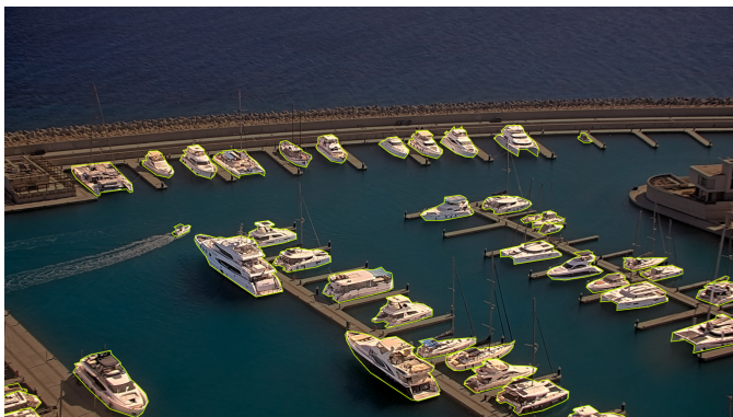
Fig. 4. Example of a manually curated segmentation annotation used to create object-detection labels. The annotation protocol focuses on visible vessel structures while excluding thin or ambiguous elements such as masts and railings.
