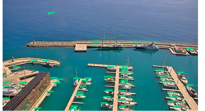
Fig. 6. Example prediction from the live PTZ camera feed using the trained YOLO26-m detector. All boats within the marina are detected as well as a small boat on the horizon outside the marina.
