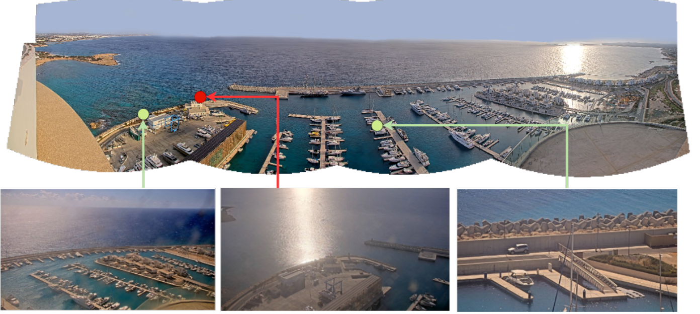
Fig. 5. Representative frame-to-panorama localization success and failure cases. Green lines show SIFT-FLANN results and red lines show SuperPoint-LightGlue results. The dots indicate recovered panorama locations, while markers outside the panorama indicate failed localization cases where not enough reliable keypoints were detected. The bottom images show examples where one of the methods failed under challenging visual conditions.
