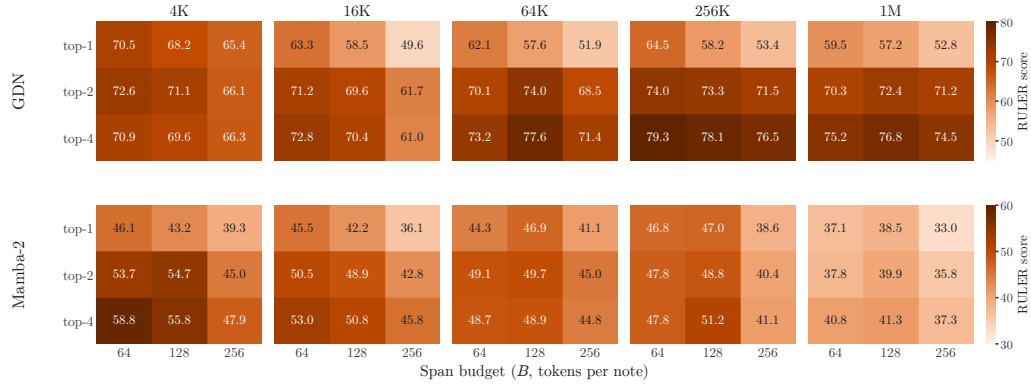
Figure 11: Joint effects of span and replay budgets. Six-task mean RULER accuracy (%) for NB-TF on GDN (top) and Mamba-2 (bottom), at context lengths from 4K to 1M. Each heatmap varies the span budget B \in \{64, 128, 256\} across columns and replay budget R \in \{1, 2, 4\} across rows. Longer spans do not consistently improve accuracy; their benefit depends on the replay budget and backbone.
