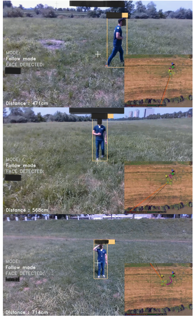
Fig. 7: Outdoor evaluation of the proposed fusion algorithm in a restricted environment. Bottom Right: UAV geolocation and person location (yellow pin), with UAV path (purple line). The proposed method successfully tracks the target person in various lighting conditions and eliminates outliers, confirming its suitability for real-time applications in SAR operations.
