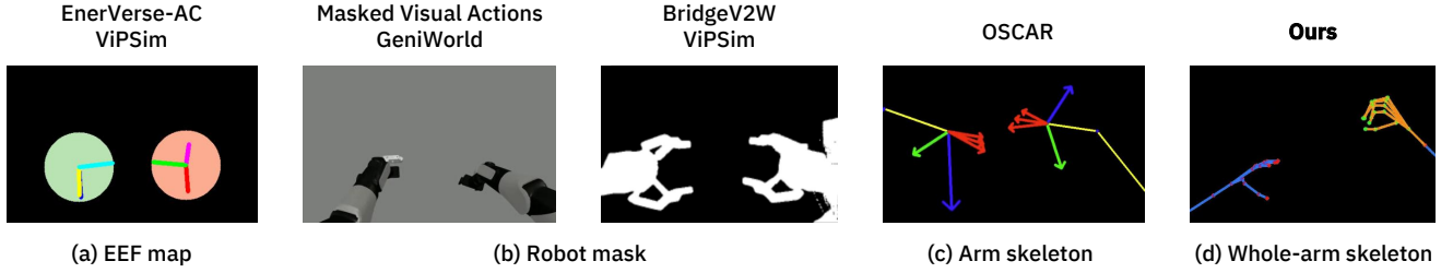
Figure 2: Geometric cues in visual action representations. (a) End-effector maps provide local pose guidance. (b) Robot masks represent projected occupancy. (c) Arm skeletons depict the kinematic chain and gripper-state cues. (d) Our camera-aligned, URDF-rendered skeleton videos provide whole-arm motion guidance with gripper or hand-state cues. Method names indicate representative approaches.
