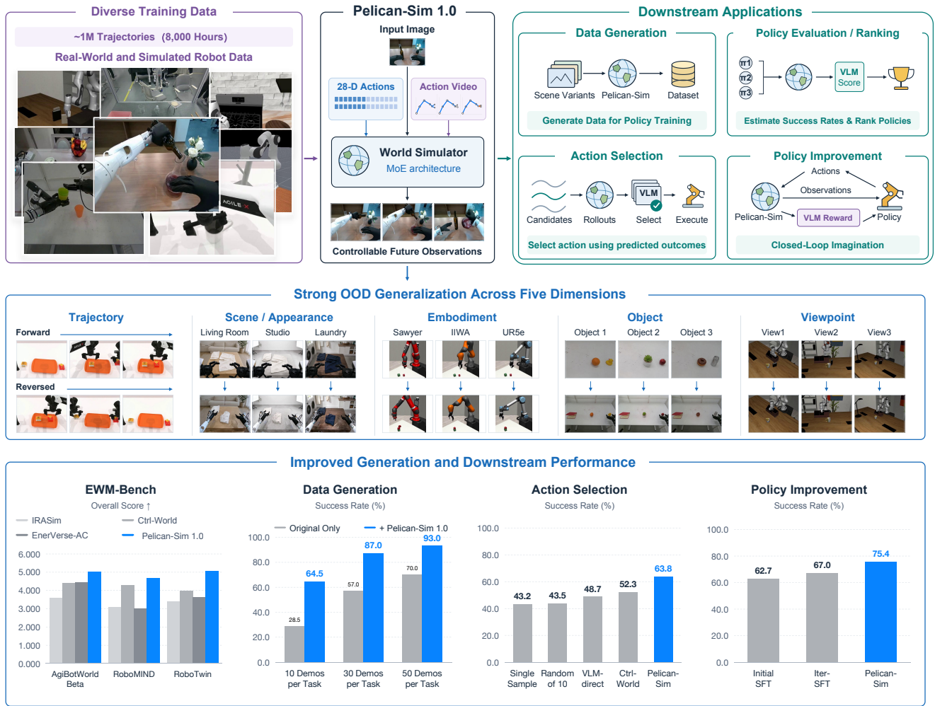
Figure 1: Overview of Pelican-Sim 1.0. Top: Trained on approximately one million real-world and simulated trajectories, Pelican-Sim 1.0 predicts future observations from an initial RGB image, unified 28-dimensional action values, and camera-aligned action videos using a Video DiT with sparse MoE layers. Four downstream applications are illustrated: data generation for policy training, policy evaluation and ranking, action selection, and policy improvement. A fine-tuned VLM evaluator supplies success estimates, candidate scores, and rewards for the latter three applications, respectively; policy improvement uses closed-loop imagined interaction. Middle: Qualitative examples illustrate generalization across five dimensions: reversed trajectories, edited scenes and object variants, held-out robot embodiments, and novel viewpoints. Bottom: Adapted EWM-Bench overall scores summarize generation performance. Separate RoboTwin studies evaluate data generation through demonstration augmentation (Data Generation), action selection, and policy improvement against their respective baselines.
