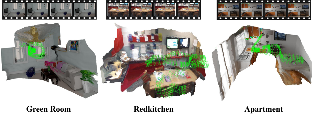
Figure 1: Robust Online 3D Reconstruction. Given a stream of RGB images as input, our BAT3R framework enables dense 3D reconstruction in an online, continuous manner, estimating both camera parameters and dense 3D geometry with each incoming frame.
