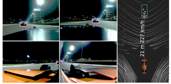
Fig. 1. UNIMORE Racing’s Dallara EAV-24 competing in the 2025 A2RL at the Yas Marina F1 Circuit. Left: detections from four cameras (pink). Right: Bird’s-Eye View showing LiDAR detection (blue) and RADAR detections (green), together with the estimated distance and velocity of the opponent.
