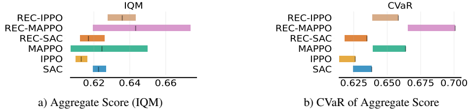
Figure 3: Aggregate Performance Analysis of Control Algorithms. This figure presents a consolidated view of algorithm performance across all evaluation scenarios. (a) The IQM of the aggregate score, where lower is better. IPPO achieves the best average performance. (b) The CVaR of the score highlights worst-case outcomes, again showing IPPO’s superiority and indicating robust performance. The wide confidence intervals for MAPPO in both (a) and (b) reveal its high sensitivity to random seeds.
