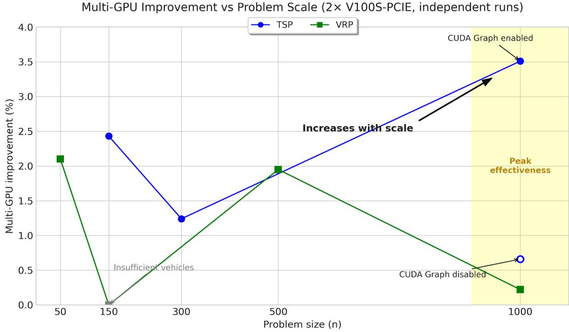
Figure 8: Multi-GPU improvement across problem scales. TSP shows increasing benefit with scale, reaching 3.51% at  $n=1000$  (CUDA Graph enabled). CUDA Graph configuration significantly affects effectiveness (3.51% vs 0.66%). VRP effectiveness depends on both scale and problem feasibility.
