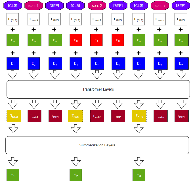
Fig. 2: Overview for the architecture of the SaraBERT model
