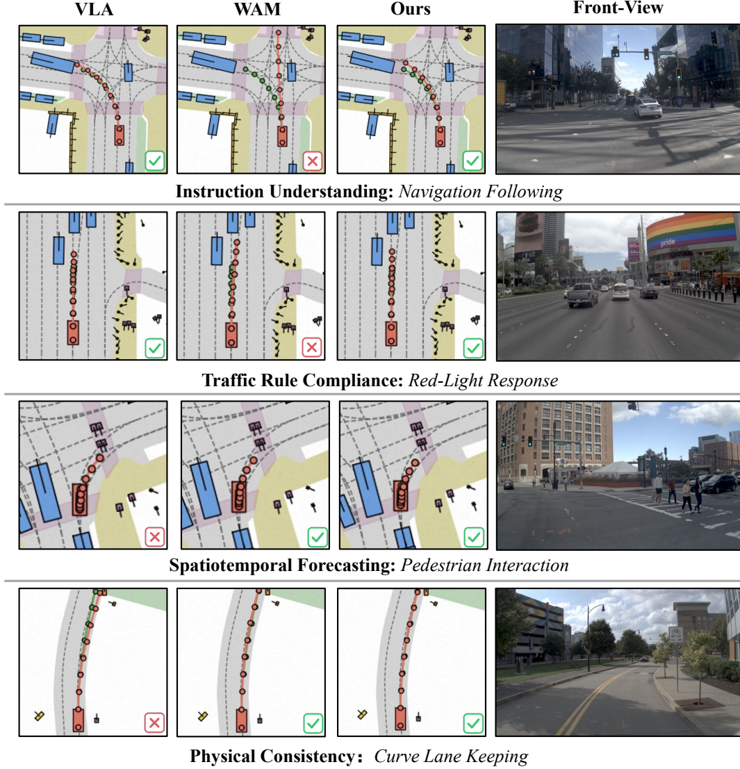
Figure 5: Qualitative comparison of VLA-only, WAM-only, and Ours in representative scenarios. Ours produces robust trajectories under semantic constraints and dynamic interactions by combining the two pathways at the action-token level.
