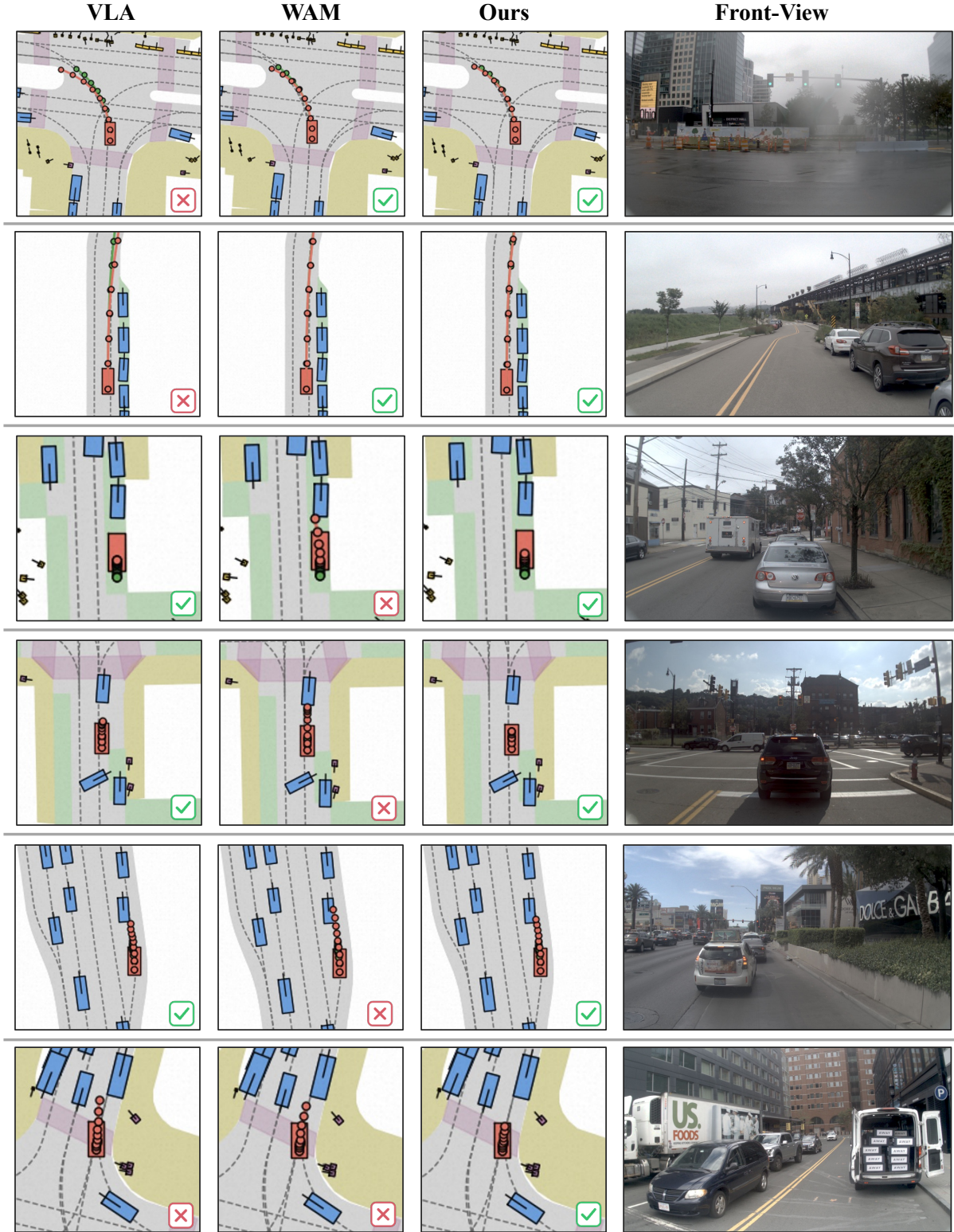
Figure 6: Additional qualitative comparisons among VLA-only, WAM-only, and BrainWAM. Each row presents the predicted trajectory in the BEV representation and the corresponding front-view image. The first two rows show cases where WAM-only succeeds while VLA-only fails, whereas Rows 3–5 show the opposite. In the last row, both single-branch models fail, while BrainWAM still produces a reasonable trajectory. These examples demonstrate the complementary strengths of semantic priors and predictive dynamics, as well as the effectiveness of their action-space coordination in BrainWAM.
