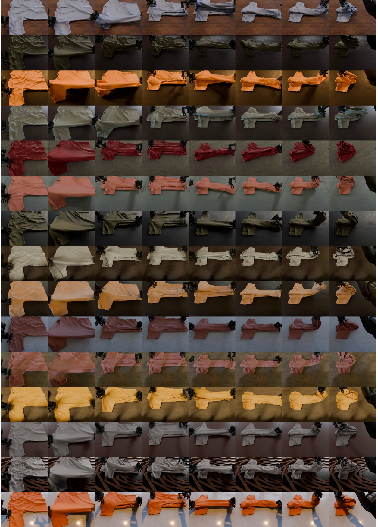
Figure 13. Synthetic generated data of T-shirt folding. Each row shows a temporally sampled trajectory with randomized textures, illustrating the visual diversity generated by our pipeline.
