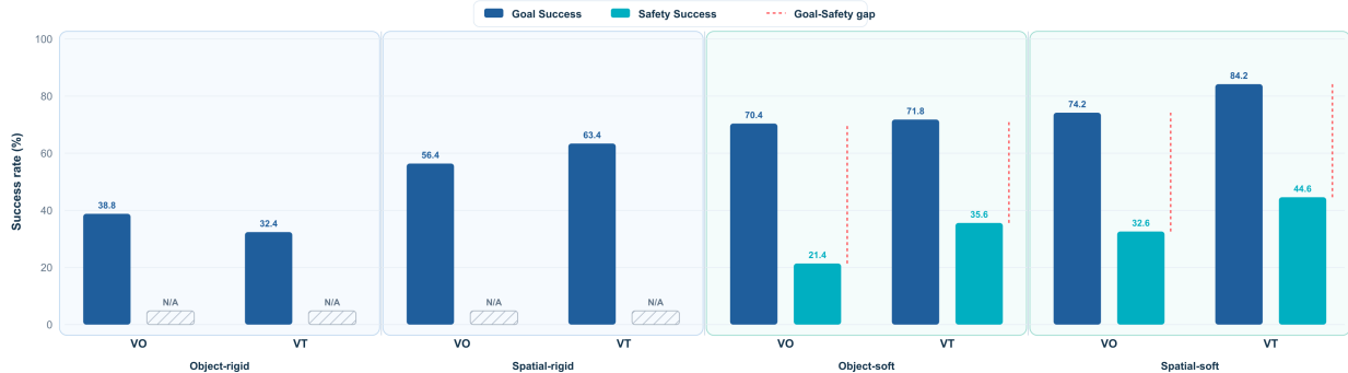
Figure 4 Goal Success and Safety Success across rigid and deformable task suites. Goal Success measures task completion, while Safety Success further requires satisfying physical safety constraints. For rigid suites, deformation-based safety constraints are not applicable and are marked as N/A. For soft suites, the gap between Goal Success and Safety Success indicates unsafe goal completions caused by excessive deformation, dropping, or unstable contact.
