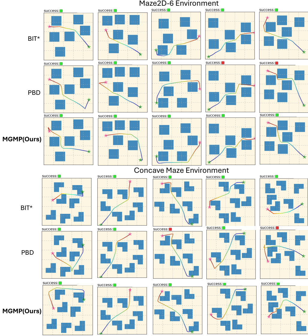
Figure 7: Qualitative results on unseen obstacle layouts in Maze2D. We compare BIT*, PBD, and MGMP on Maze2D-6 and Concave Maze2D. MGMP generates collision-free trajectories that reach the goal while avoiding unseen obstacle placements.
