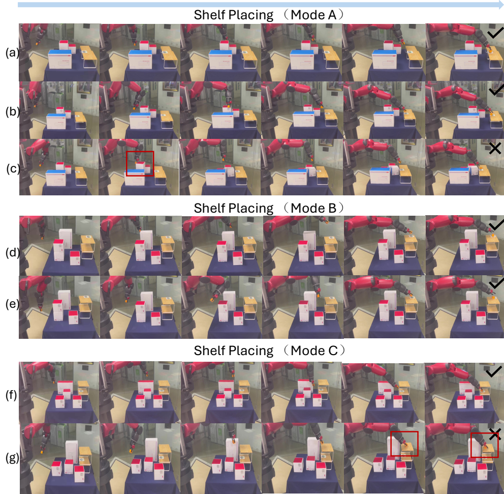
Figure 19: Qualitative results for the real-world shelf-placing task under three target shelf modes. MGMP successfully generates obstacle-avoiding trajectories that reach valid release poses. Failure cases are mainly caused by obstacle collisions or unsuitable approach trajectories that prevent successful placement.
