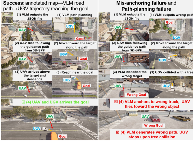
Fig. 4. Representative episodes. Success: the annotated map drives a VLM road path that the UGV tracks to the goal, with the UAV and UGV both arriving. Mis-anchoring failure: the UAV’s VLM anchors onto a similar but wrong truck and flies toward the wrong object. Path-planning failure: the UGV’s VLM plans a path that collides with a tree, stalling the UGV.
