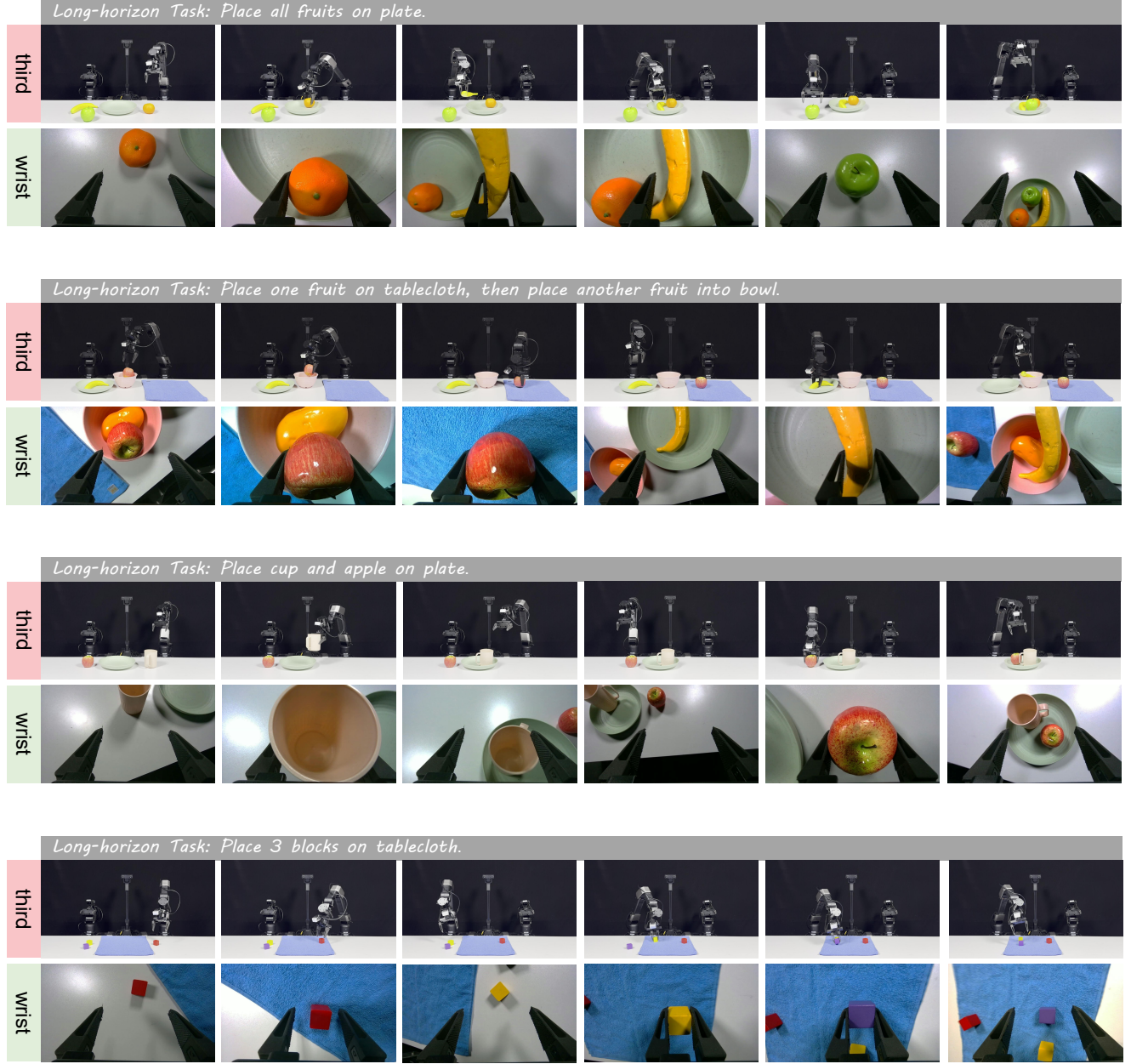
Figure 8. Qualitative results of OptimusVLA on Real-World. From top to bottom, we illustrate four Long-horizon Tasks : Place all fruits on plate , Place one fruit on tablecloth, then place another fruit into bowl , Place cup and apple on plate , and Place 3 blocks on tablecloth . Here, third denotes third-person view images, while wrist denotes images captured from the robot’s wrist-mounted camera.
