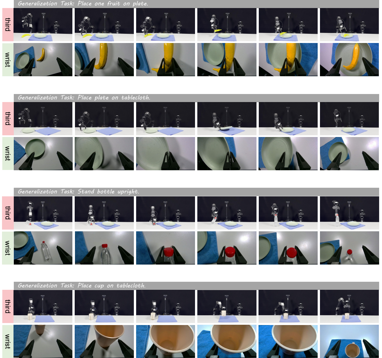
Figure 7. Qualitative results of OptimusVLA on Real-World. From top to bottom, we illustrate four Generalization Tasks : Place one fruit on plate , Place plate on tablecloth , Stand bottle upright , and Place cup on tablecloth . Here, third denotes third-person view images, while wrist denotes images captured from the robot’s wrist-mounted camera.
