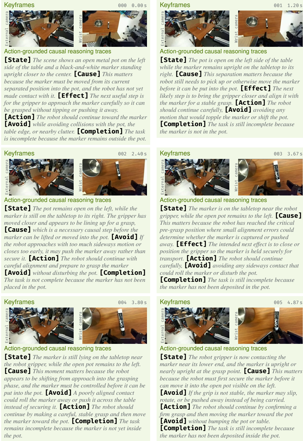
Figure 10 Full natural-language reasoning annotations for “Put the marker in the pot,” with synchronized external- and wrist-camera views. Part 1: labeled keyframes 000–005.
