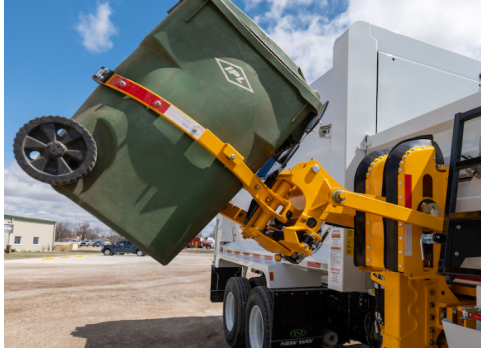
(a) Automatic side-loader in operation
