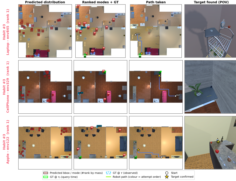
Figure 8: Representative successful ObjNav episodes with FlowMaps, set 1. Each row shows the predicted samples, ranked clusters, executed trajectory, and final target confirmation view.
