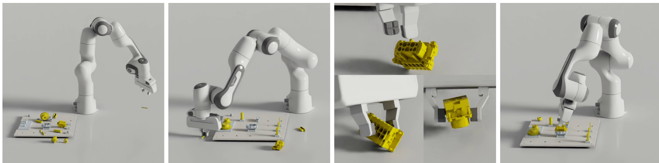
Fig. 1. Emergent multi-component assembly with a single policy. Trained with a binary task reward, AlphaNIST learns to select, grasp, reorient, and assemble diverse components, while autonomously sequencing multiple assemblies within a single episode. Shown are snapshots from a ten-component assembly sequence.
