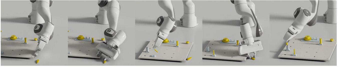
(a) Bring USB-A closer, assemble the 8 mm rod, then return
