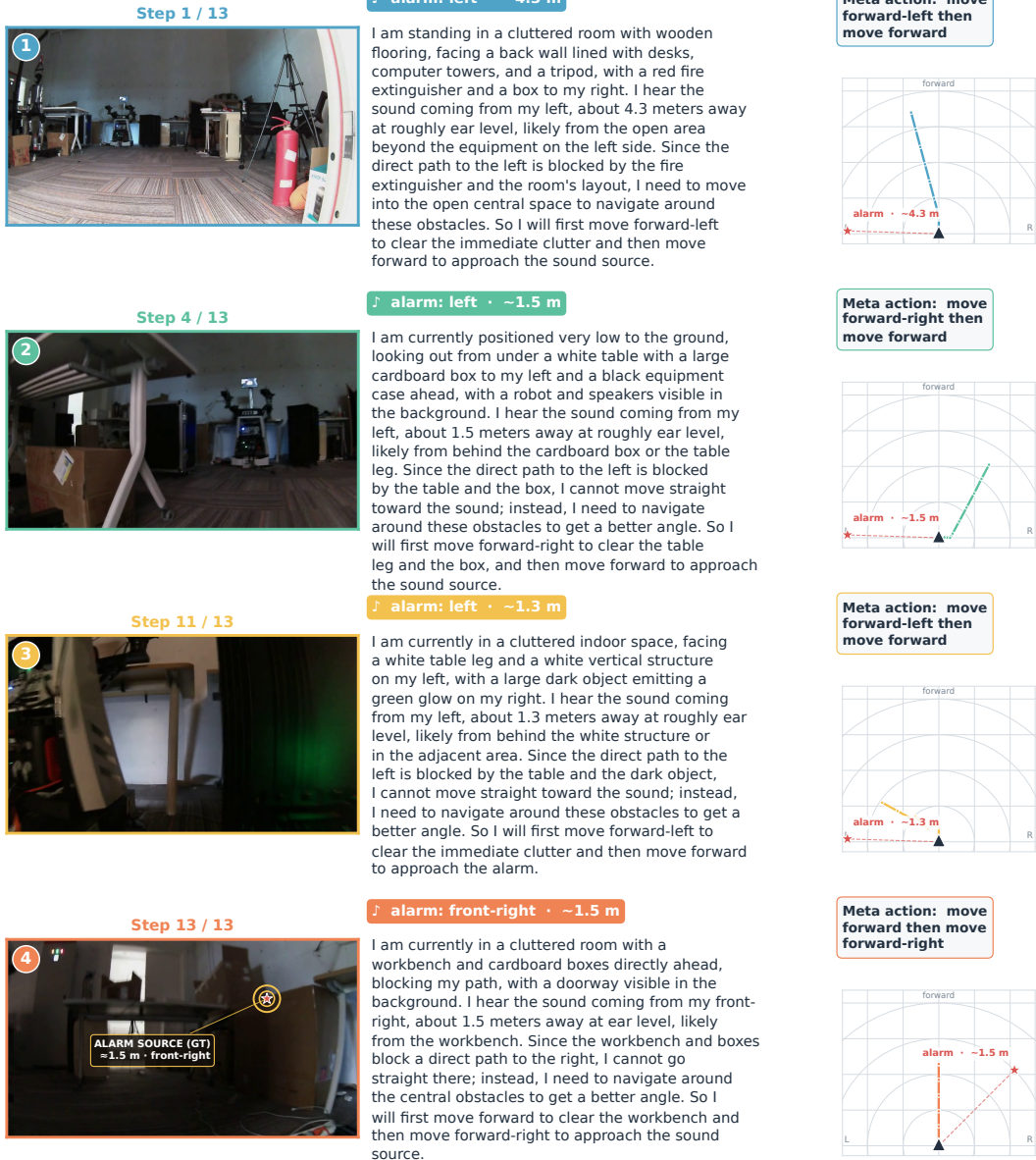
Figure 20: Qualitative example of OmniEcho deployed on a physical robot for sound-guided navigation. The robot progressively localizes and approaches an initially out-of-view alarm by jointly reasoning over egocentric spatial audio and visual observations while navigating around obstacles.
