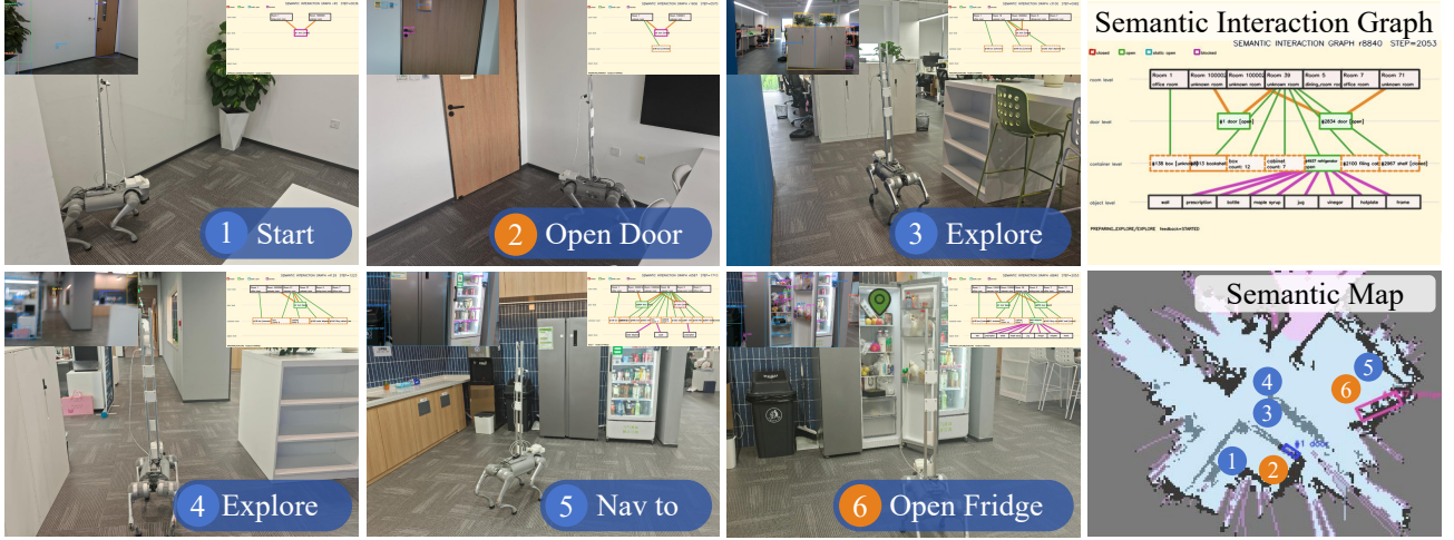
Figure 5: Real-world navigation to find an apple with Go2. The robot explores and navigates to a refrigerator, with human-assisted door and refrigerator opening. Insets show observations and interaction graphs; map markers indicate navigation (blue) and interaction (orange).
