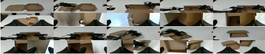
Figure 14: Real-world visualizations of Folding Box for the four WAM interfaces. Selected frames show the progression from a flat cardboard box to folding its walls and manipulating its flaps.
