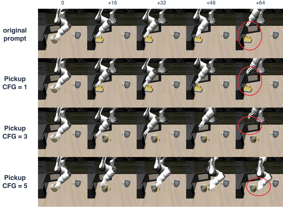
Figure 3: Effect of the guidance scale on recovery predictions. All branches start from the same trigger state and the corrective instruction “pick up the cup”.
