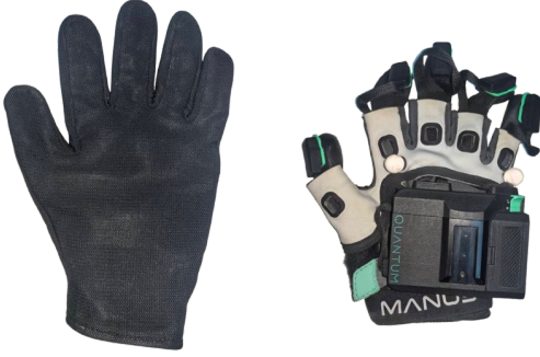
Figure 6: Hardware for human data collection. Left: the Jujiao tactile glove. Right: the Manus Quantum MetaGlove.
