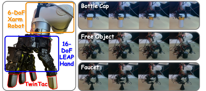
Figure 5: DexMani real-world deployment. The sequence shows closed-loop execution at 20 Hz in the real world.
