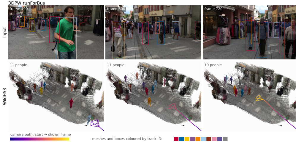
Figure 11: Crowded in-the-wild reconstruction on 3DPW downtown_runForBus. Top: input and persistent tracks. Bottom: metric scene, camera trajectory and bodies colored by identity. The sequence contains 14 tracks over 10 s, with 10 to 11 people reconstructed per frame.
