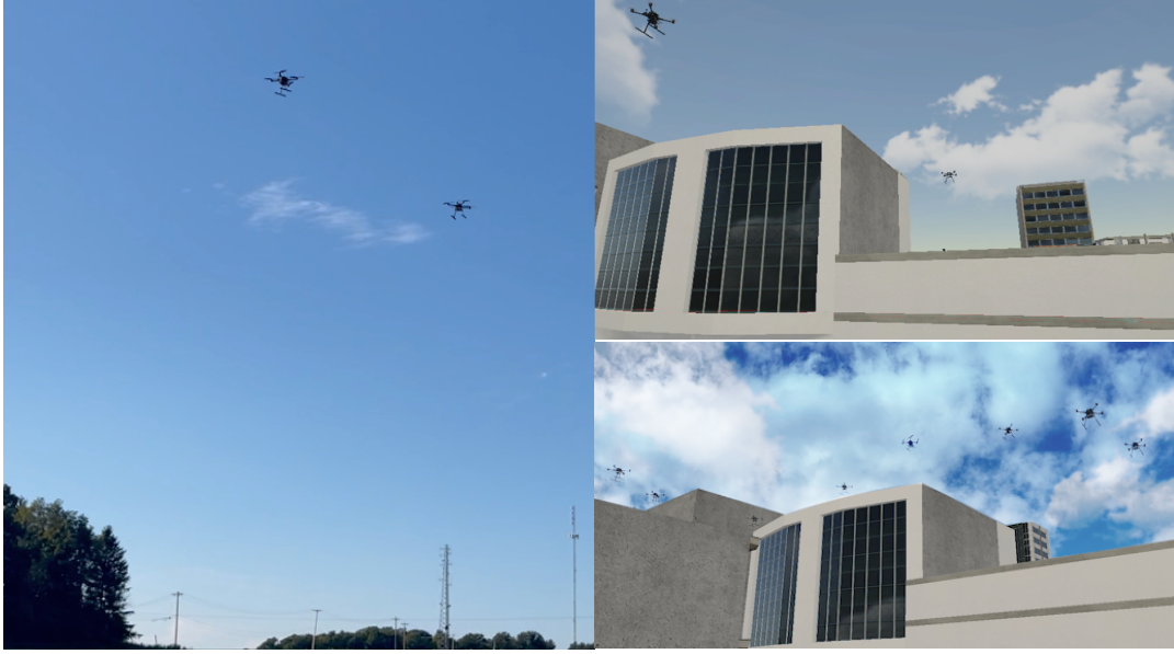
Fig. 1. Real-time field-anchored evaluation infrastructure. Left: physical multi-drone field operation. Upper right: corresponding field-synchronized real-time simulation view of the 1:1 urban operating environment. Lower right: hybrid operation coupling live hardware nodes with real-time simulated traffic, urban context, and scenario constraints. The stack exercises operational complexity around physical flight in real time, grounding communication and tactical-coordination results in closed-loop hardware behavior.
