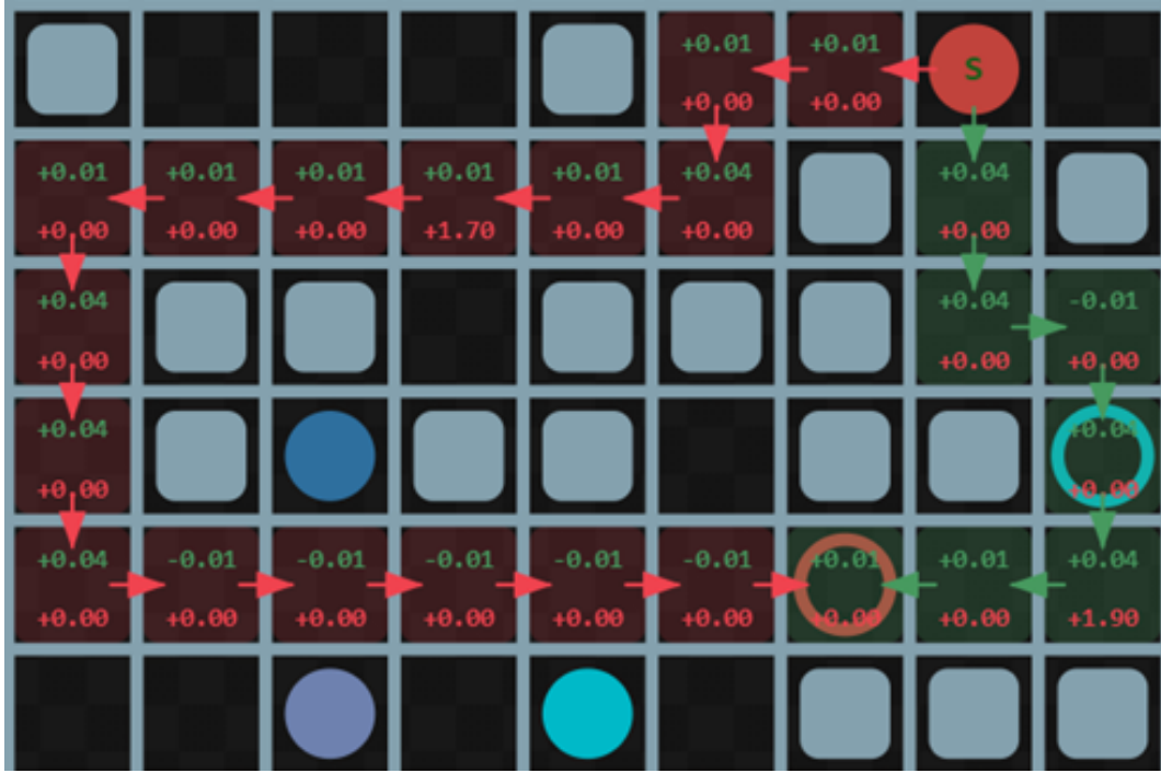
Figure 9: Two sample trajectories captured during an episode, along with the rewards the agent is expected to receive. All neighboring agents remain stationary in this example while the red agent traverses toward its goal. Green values indicate the learned reward (ARMS) while red values indicate the original sparse reward. Since the agent has already partially progressed along its path, the sparse reward accumulated over the previous 20 timesteps is received at timestep 5. The rewards are scaled \times 10 for visual convenience. In the shorter trajectory, the agent reaches the goal exactly at timestep 7, causing the accumulated sparse reward to be delivered two cells away from the goal. The sum of ARMS' reward at the shorter path is +0.20 while the longer path +0.22 , indicating that higher reward can be accumulated when taking shorter paths.
